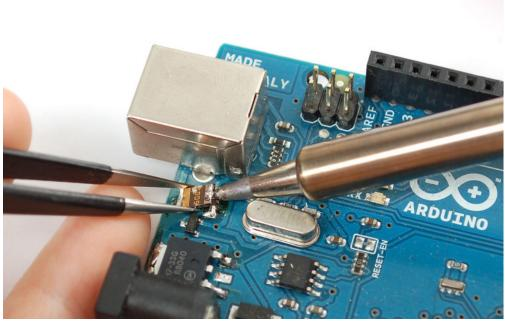
Clip the diode short and bend the leads over. Solder the side without a stripe (anode) to the old fuse pad, nearest the board edge. Solder the striped end (cathode) to the right hand leg of the regulator.
