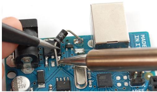
That's it! You are now 3.3V powered. This is a little lower than the power/frequency specification for the AVR chips since they ought to have about 3.6V to run 16Mhz but its *probably* not going to be an issue since AVRs can be overclocked a little. Upgrade Arduino Hacks
